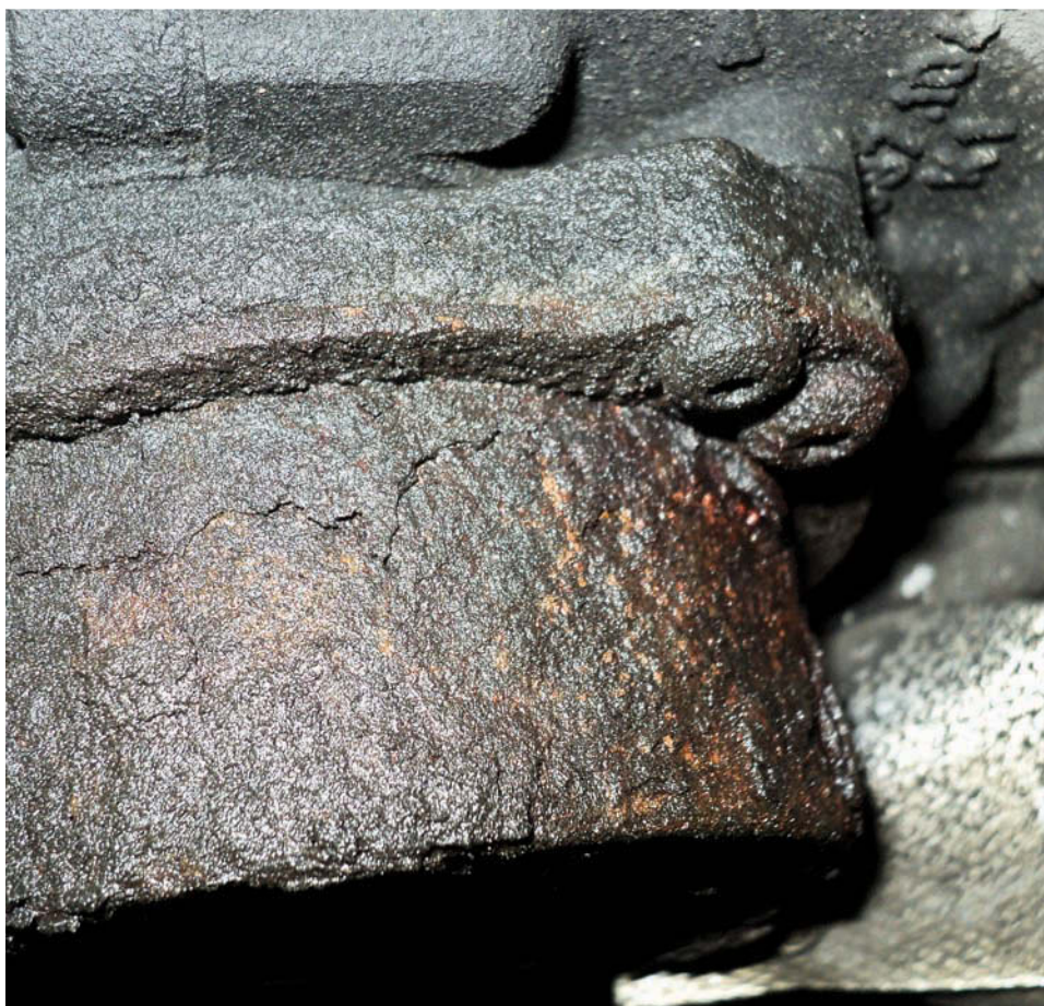
Below: A leaking tandem pump on a 2006 997
