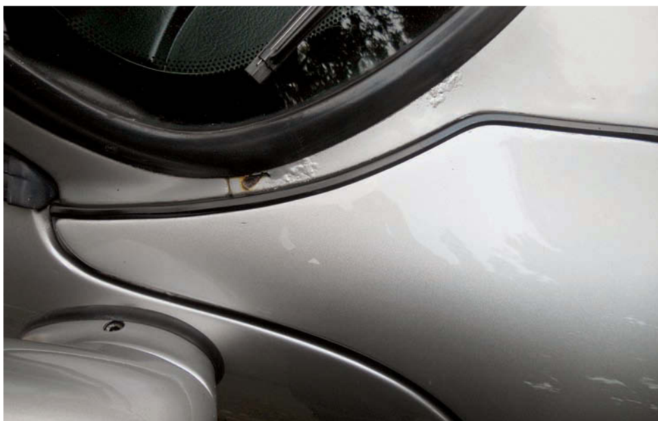
Here: Window trim corrosion on the 993 Below: 993 scuttle corrosion
