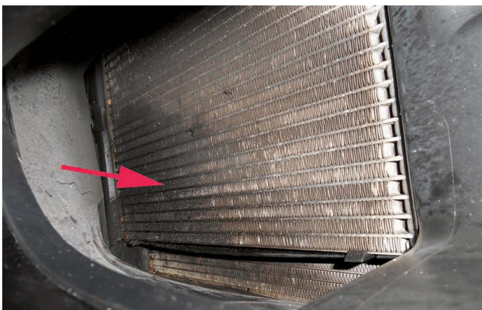
Above: Tandem pump in situ on 997 Carrera Below: Condenser leak damp patch on a 997
