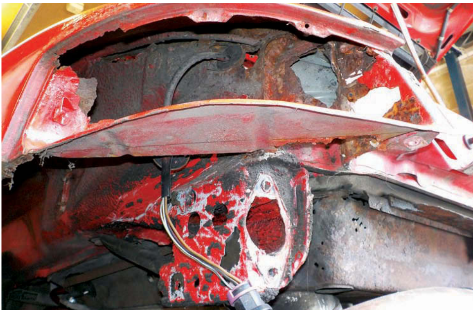
Previous page: Corrosion damage to 964 inner wing in engine bay Above: Heavy corrosion behind 964 rear light fitting Below: Severe corrosion to 964 sill and wings
